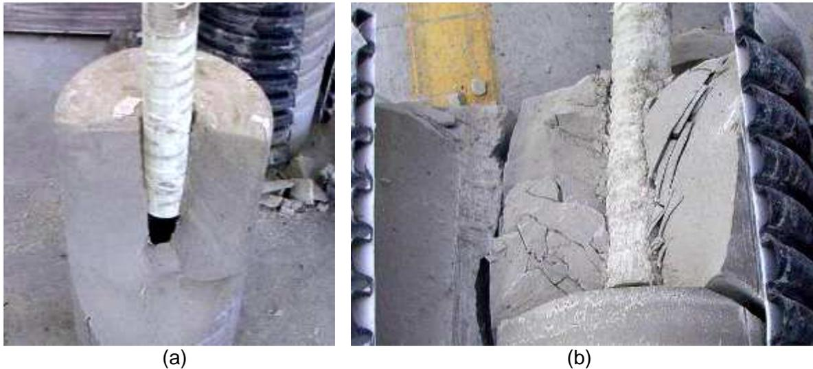
Figure 8 Pictures showing the different mechanical interaction between pipes and cement grout from laboratory pull out tests on (a) standard improved adherence (AM) and (b) corrugated (CRG) pipe samples
