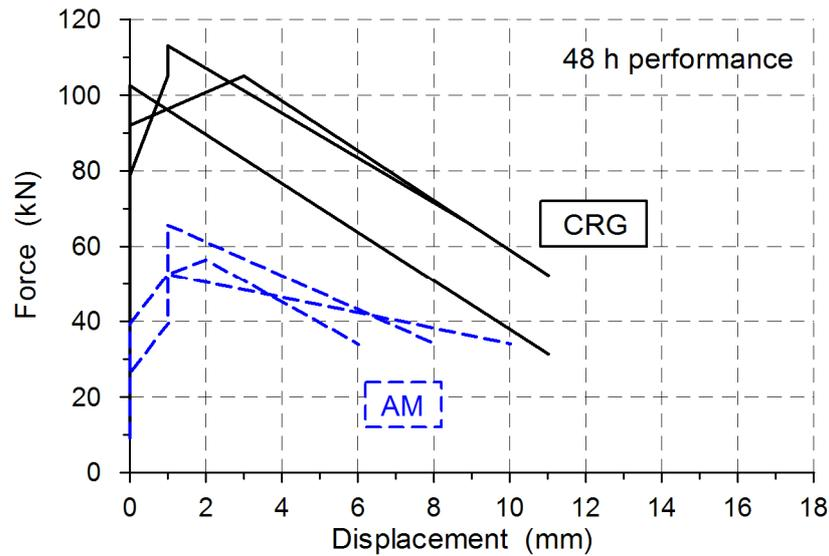
Figure 7 Results from pull out laboratory tests on standard improved adherence (AM, dashed lines) and corrugated (CRG, solid lines) pipe samples, 48 hours after grout injection (sample length = 300 mm, external diameter = 60 mm, internal diameter = 40 mm)
