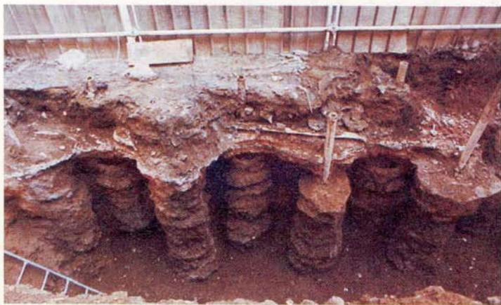
Fig. 3 Campo prove jet-grouting (particolare)
