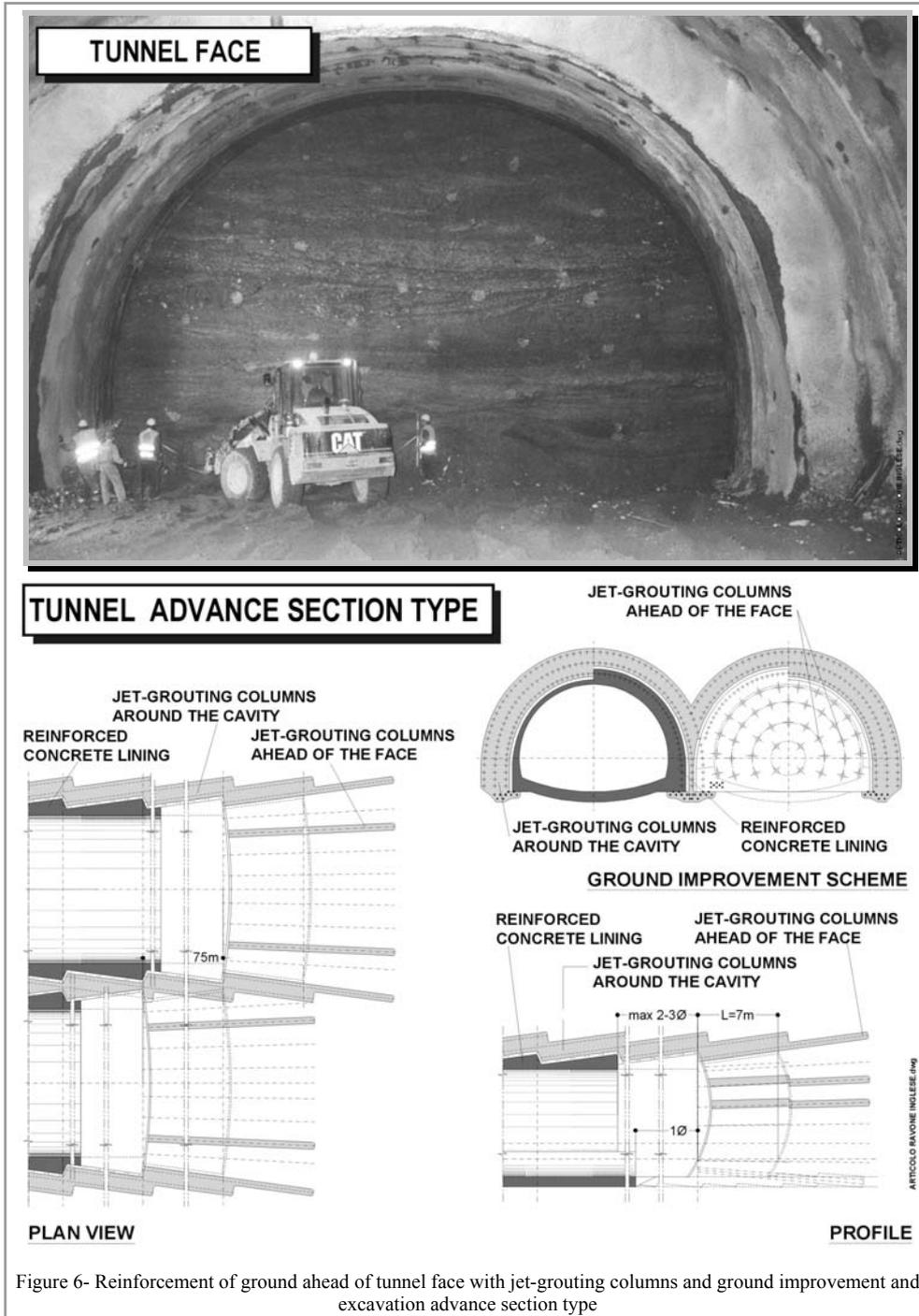
Figure 6- Reinforcement of ground ahead of tunnel face with jet-grouting columns and ground improvement and excavation advance section type
