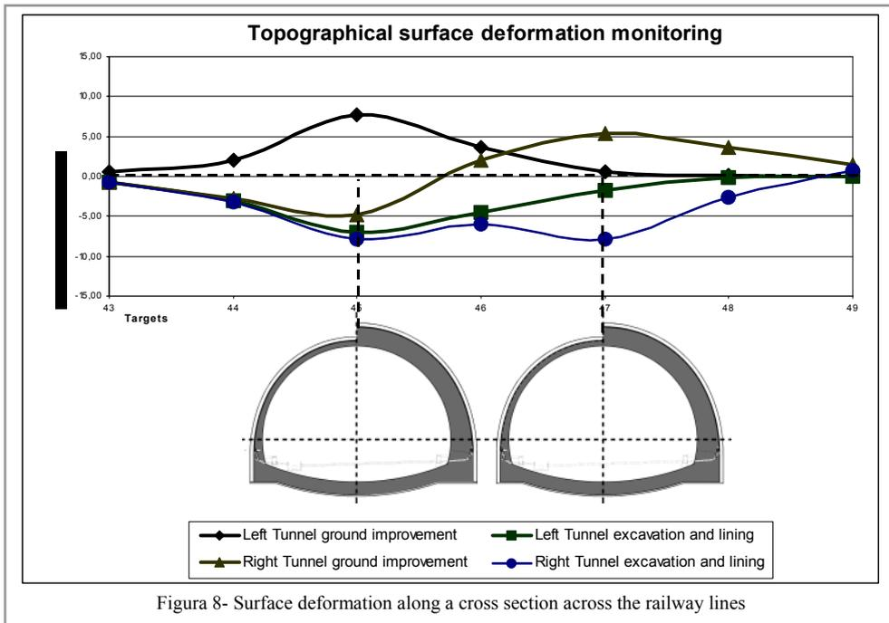
Figura 8- Surface deformation along a cross section across the railway lines
