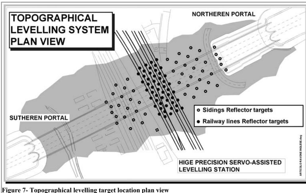
Figure 7- Topographical levelling target location plan view
