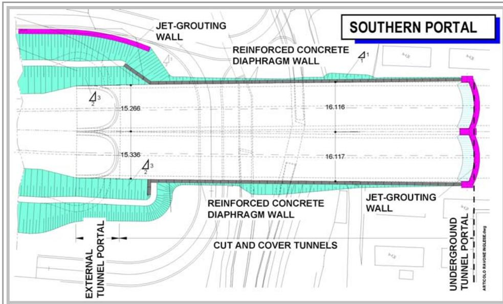
Figure 2 – SOTHERN PORTAL: diaphragm walls plan view.
