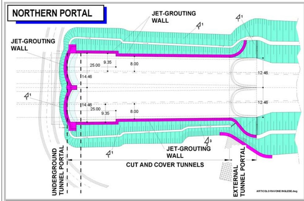
Figure 3 – NORTHERN PORTAL: diaphragm walls plan view.
