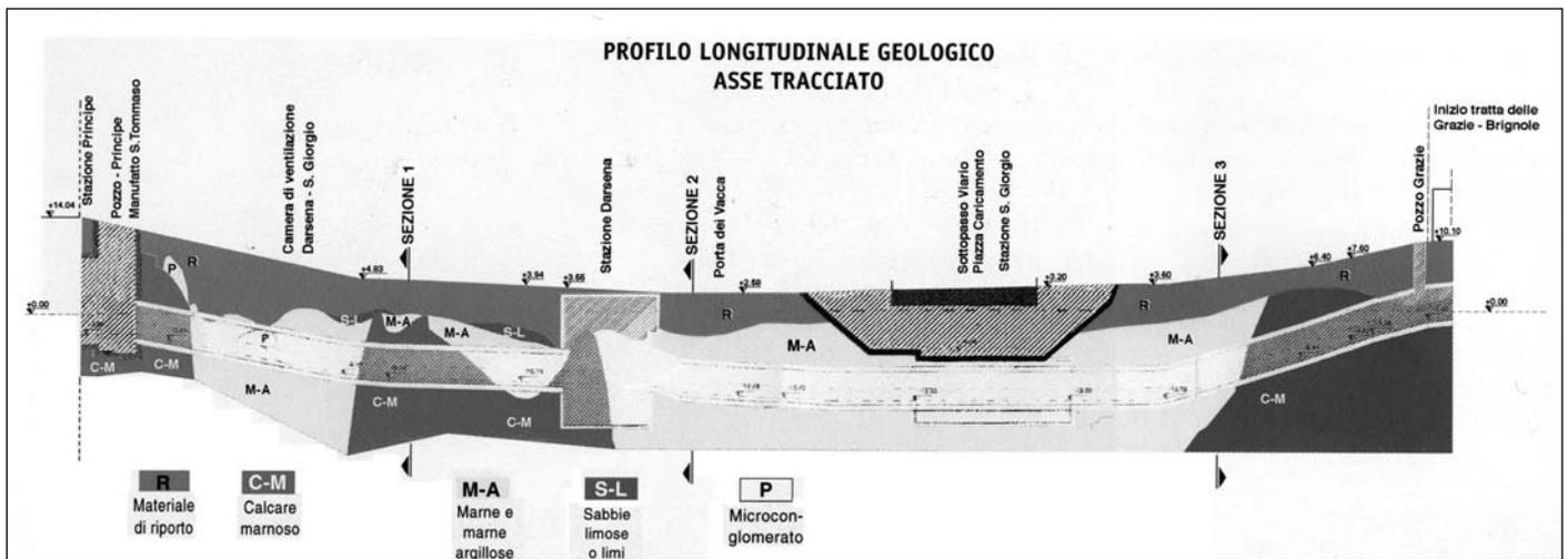
tion of buildings foundation and Genoa Fly-over Road pillars foundation along the tunnels route. Grout injection has been carried out according to MPSP (Multiple Packer Sleeved Pipe) system.
