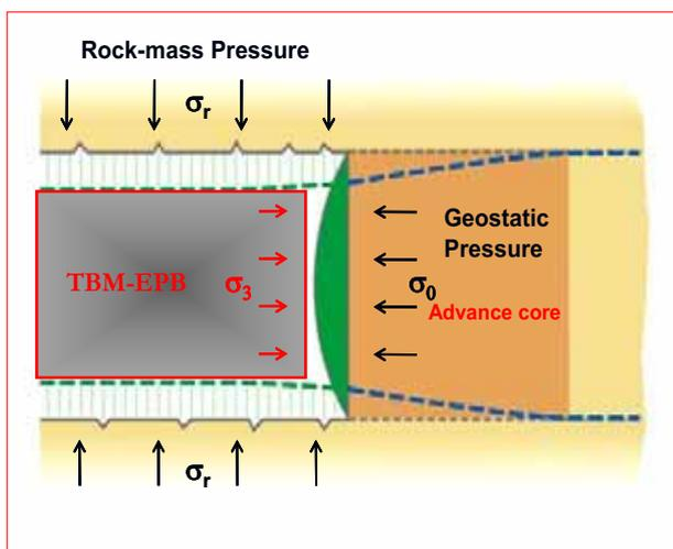
**Fig. 3** – Analysis of the deformation response
