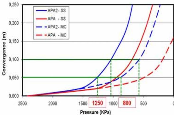
Fig. 5 - APA (H=110m) - Pressure-convergence curves
