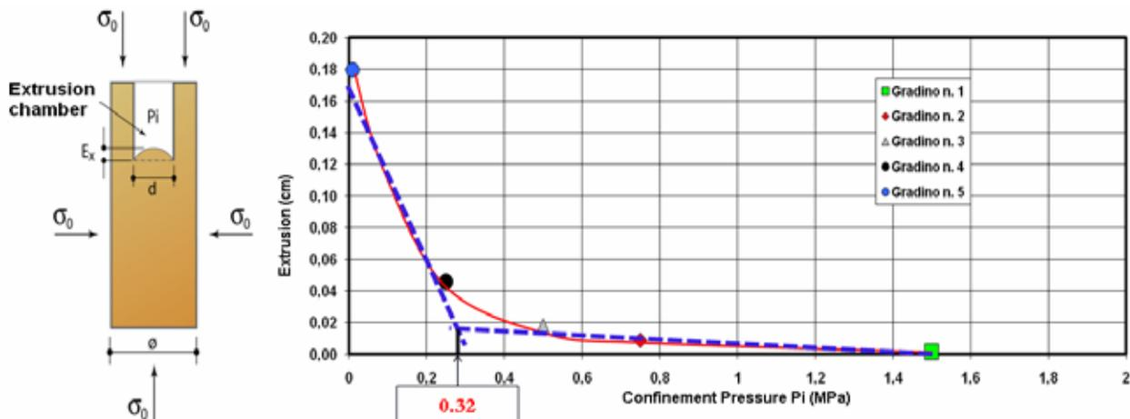
Fig. 4 – Triaxial extrusion test, Extrusion-Confinement Pressure Curve
