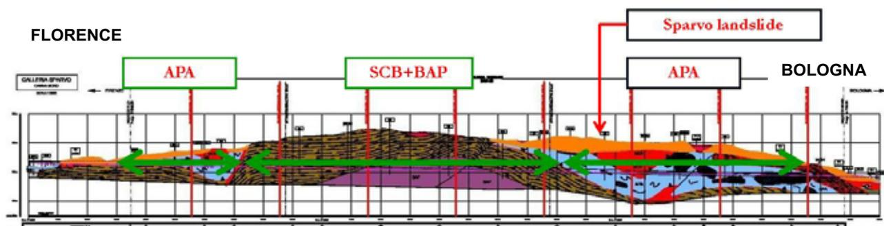
**Fig. 2** Sparvo Tunnel geological longitudinal section
