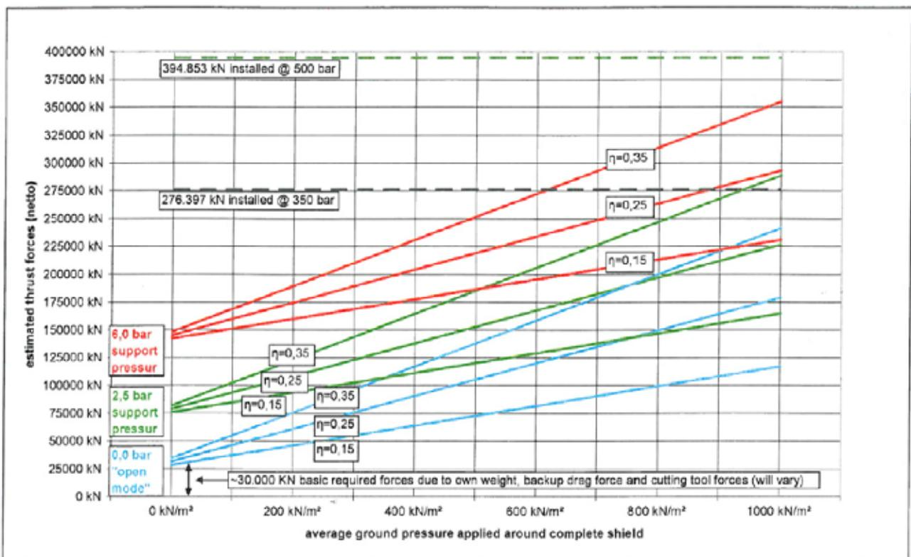
**Fig. 6** – Study of the total thrust of the TBM (Herrenknecht AG)
