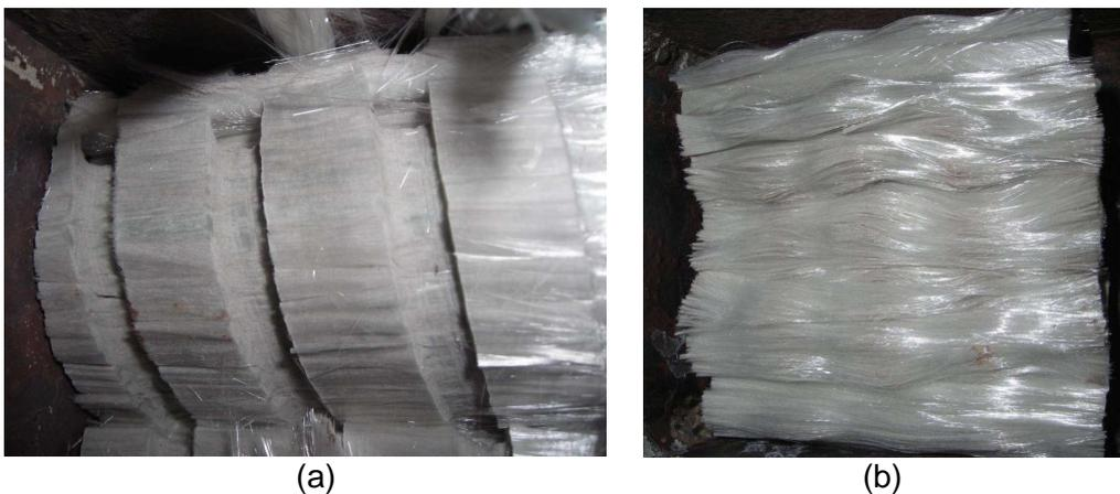
Figure 2 Glass fibre mass after heating treatment: from (a) 60/40 AM pipe with spiral groove and (b) 60/40 CRG corrugated pipe, as in Figure 1
