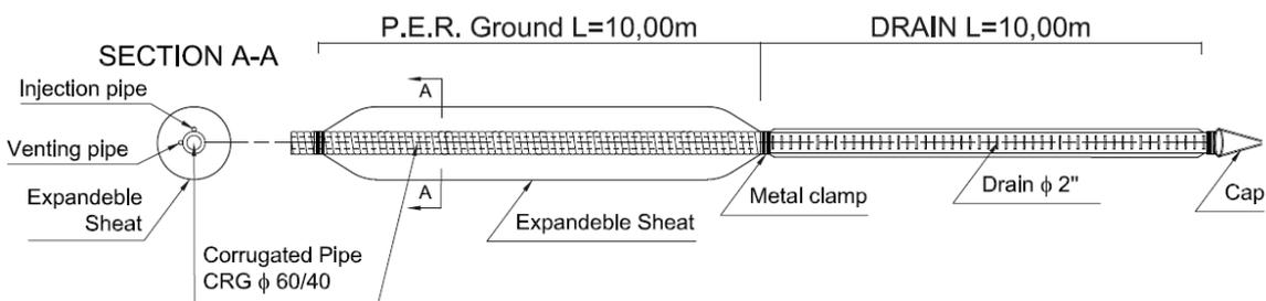
Figure 4 Soil nail for the coupled tunnel face reinforcement and drainage, as a modification of PERGround® shown in Figure 3
