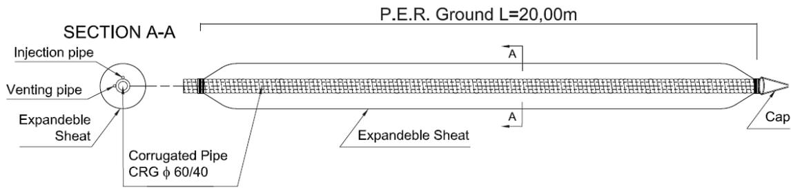
Figure 3 Soil nail for the tunnel face reinforcement (PERGround®, Elas Geotecnica S.r.L.)
