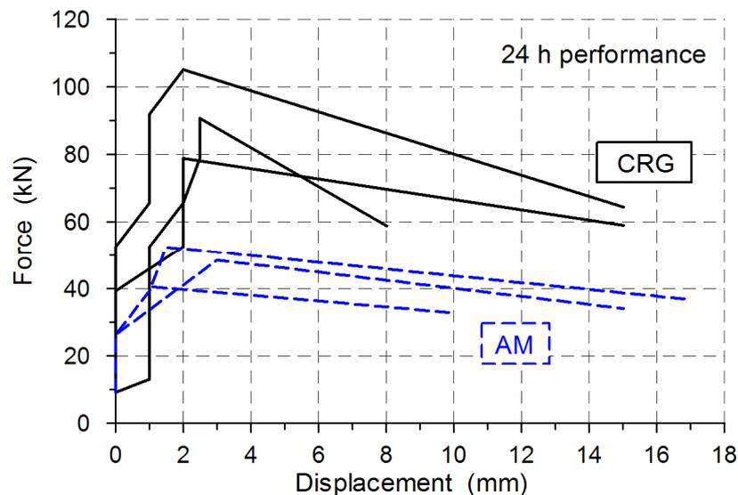
Figure 6 Results from pull out laboratory tests on standard improved adherence (AM, dashed lines) and corrugated (CRG, solid lines) pipe samples, 24 hours after grout injection (sample length = 300 mm, external diameter = 60 mm, internal diameter = 40 mm)
