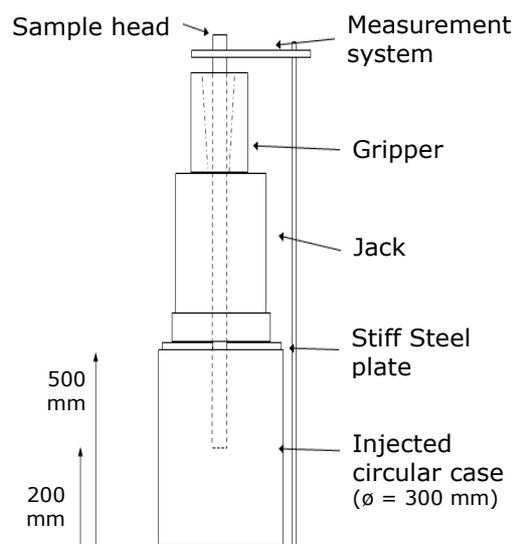
Figure 5 Set up for laboratory pull out tests on GFRP pipe samples
