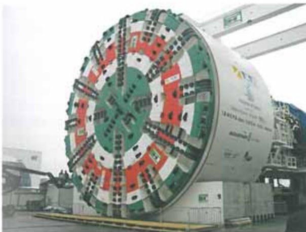
8a The Sparvo EPB TBM (named "Martina")
