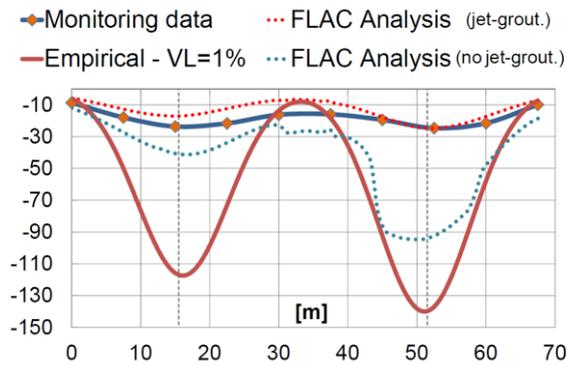
Figure 18. Ground level subsidence (mm).
