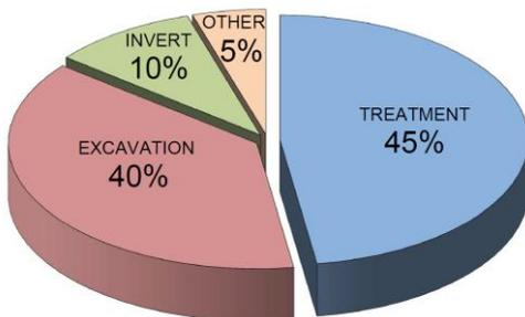
Figure 12. Section type C1b: work cycle .
