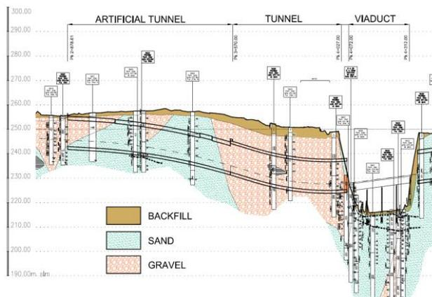
Figure 5. Tunnel geological longitudinal section (overburden 2-13 m, Ø = 19 m).
