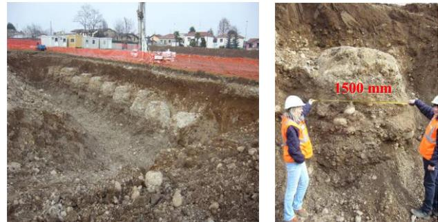
Figure 7. “Jet-grouting” field tests (1500 mm).
