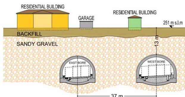
Figure 17. “Via Opificio Valle” cross-section.
