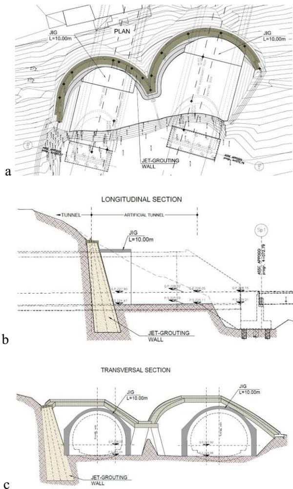
Figure 14. Portal jet-grouting wall: a) plan, b) longitudinal section, c) transversal section.
