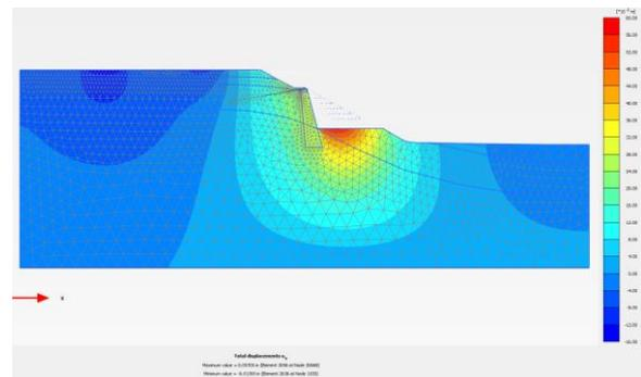
Figure 15. Numerical analysis: horizontal movements.
