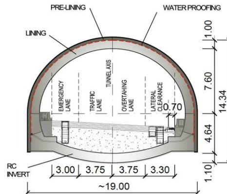
Figure 3. Tunnel section layout.
