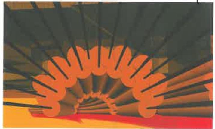
Above: Figure 2, Soil treatment around the tunnel
