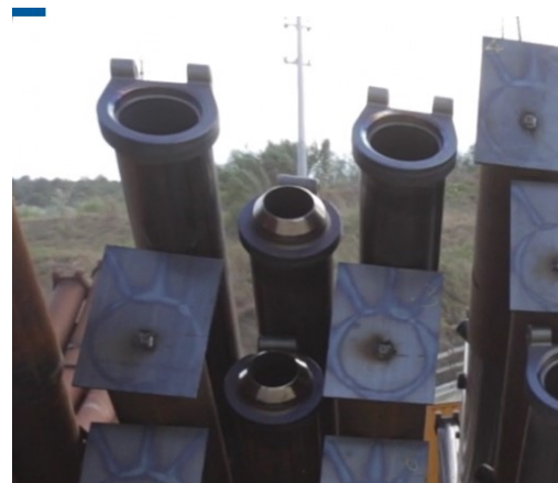
Figure 11. Tubular Arch: junction plate detail.
