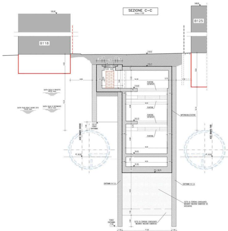
Figure 12. Section of the revised station project, with the position of the ancient wall.
