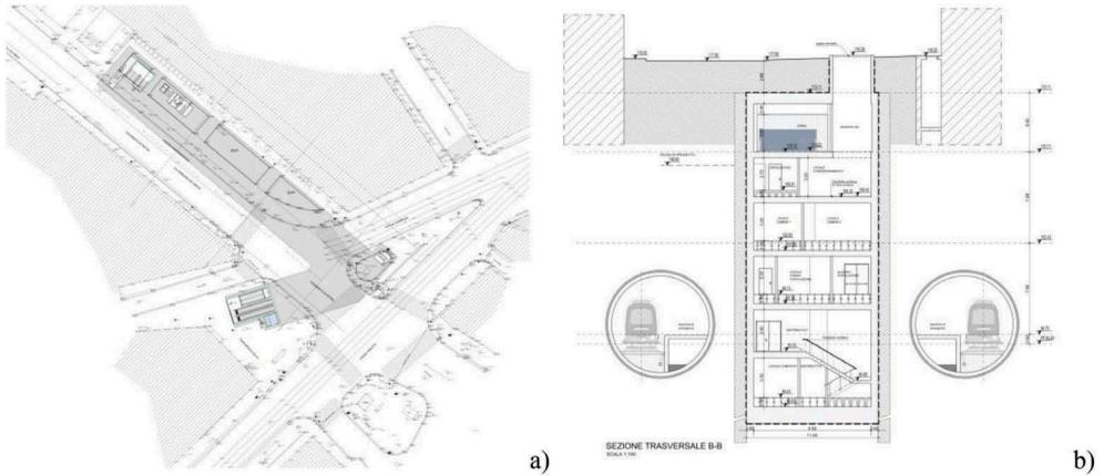
Figure 8. Original project of De Amicis Station: a) layout; b) transversal section.
