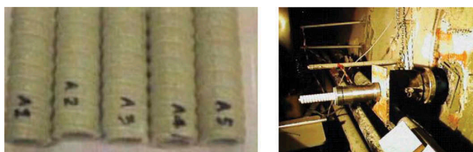
Figure 4. Corrugated ground elements and Fiber glass extraction test.
