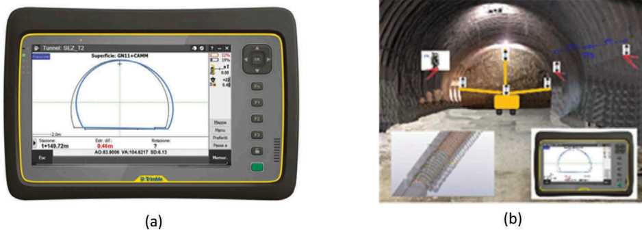
Figure 10. (a) Ekip steel rib placer topographic assistant. (b) Ekip steel rib placer topographic hardware.
