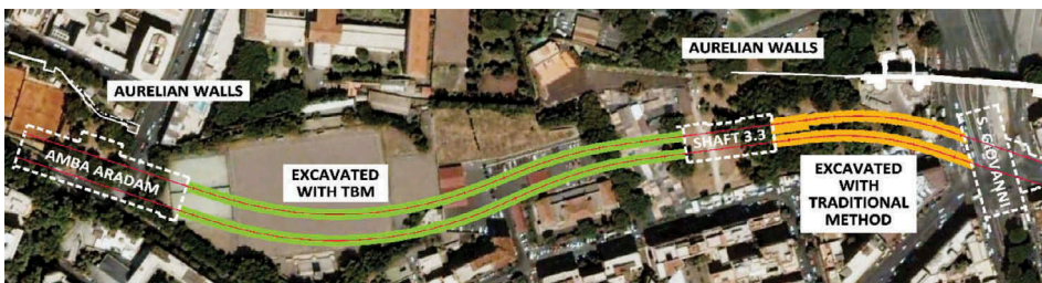
Figure 2. T3 first track between shaft 3.3 and Amba Aradam Station.
