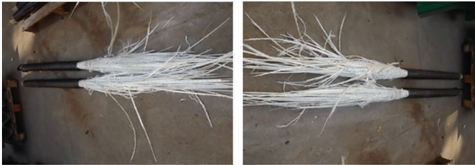
Figure 4.36 Glass fibre-reinforced polymer pipes subjected to tensile tests after failure.
