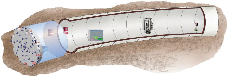
Figure 5.30 Overview of TBM position monitoring system. (Courtesy of TACS Gmbh.)
