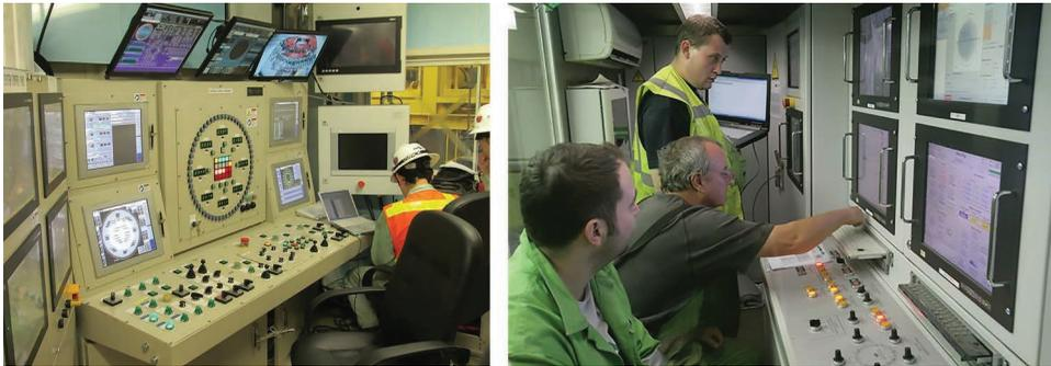
Figure 5.24 Typical TBM “control room” for monitoring data analysis. (Courtesy of Geo-data Engineering SpA.)
