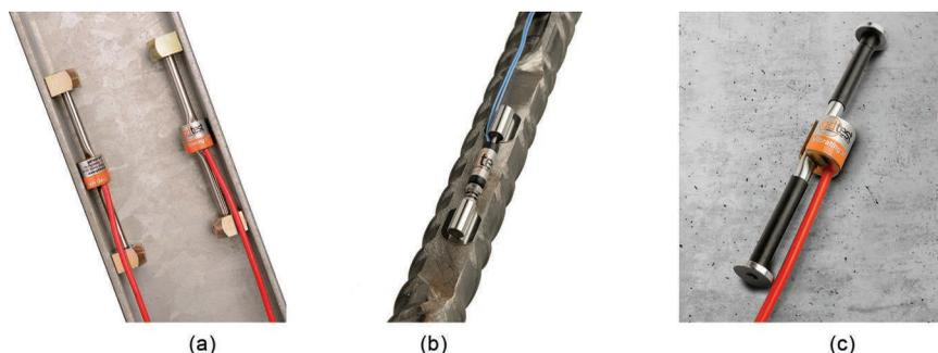
Figure 5.16 Different types of vibrating wire strain gauges: arc weldable, spot weldable and embedded. (Courtesy of GD Test S.r.l.)
