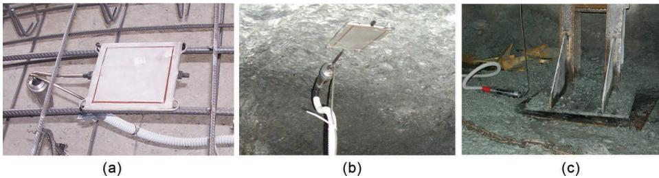
Figure 5.19 Example of different types of pressure cells and their application.
