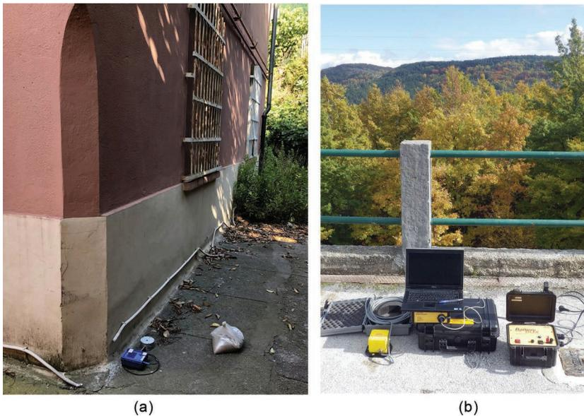
Figure 5.23 Example of vibration measuring devices. (Courtesy of Instantel Inc. and Sol-Geo S.r.l.)
