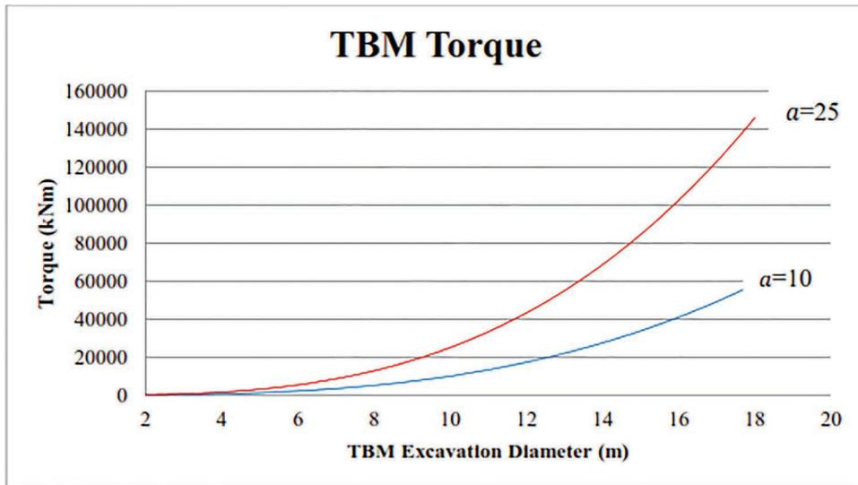
Figure 5.27 The empirical relationship between TBM's cutter head torque and TBM's diameter (Zhou & Zhai, 2018).
