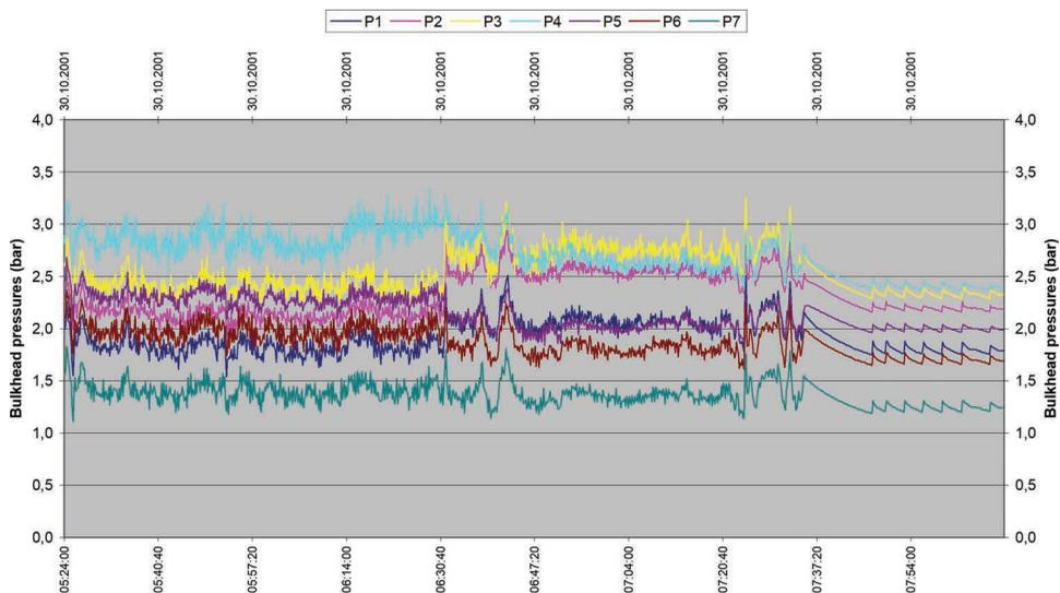
Figure 5.36 Pressure measured in pressure sensors positioned at different levels in the excavation chamber versus time. (Courtesy of Geodata Engineering SpA.)
