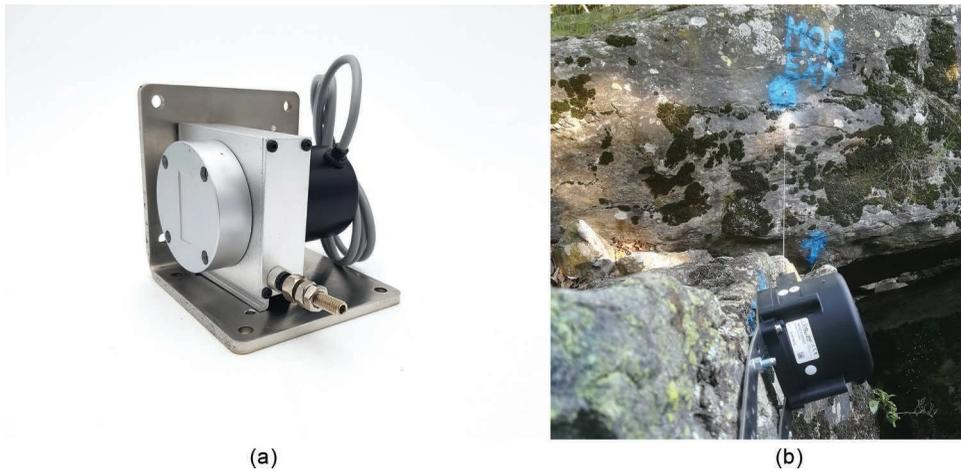
Figure 5.12 Type of surface extensometer and example of installation on a rock slope above a tunnel under construction for stability monitoring. (Courtesy of Gestecno S.r.l. and GD Test S.r.l.)
