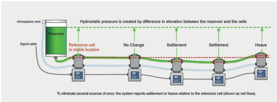
Figure 5.6 HLS functioning layout. (Courtesy of Geo-Instruments.)
