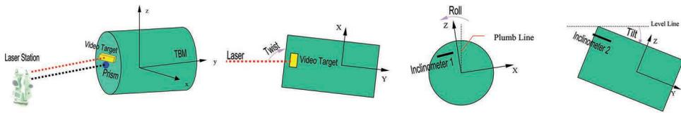
Figure 5.29 Example of working principles of TBM guidance system (Lee, 2007).
