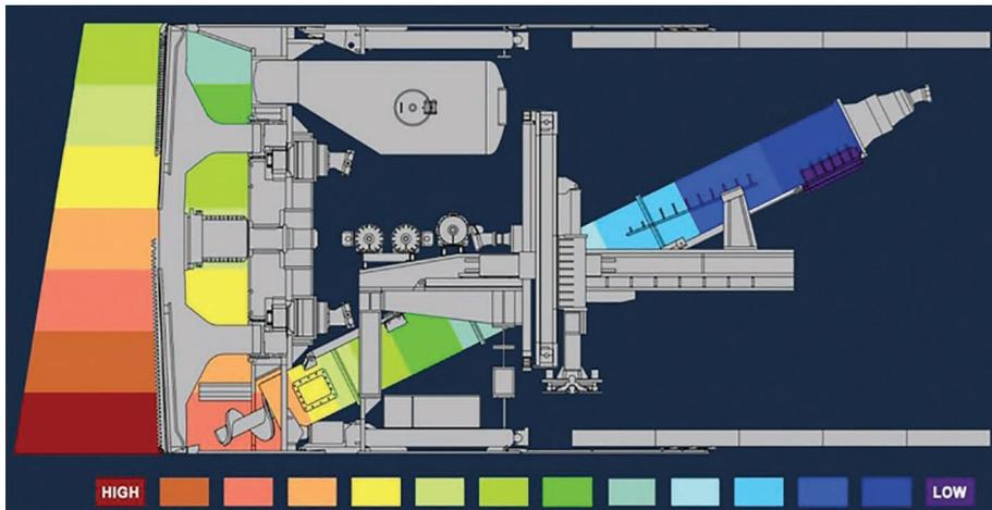
Figure 5.38 The typical (ideal) pressure distribution in excavation chamber and screw conveyor of EPB TBM (Lovat, 2012).
