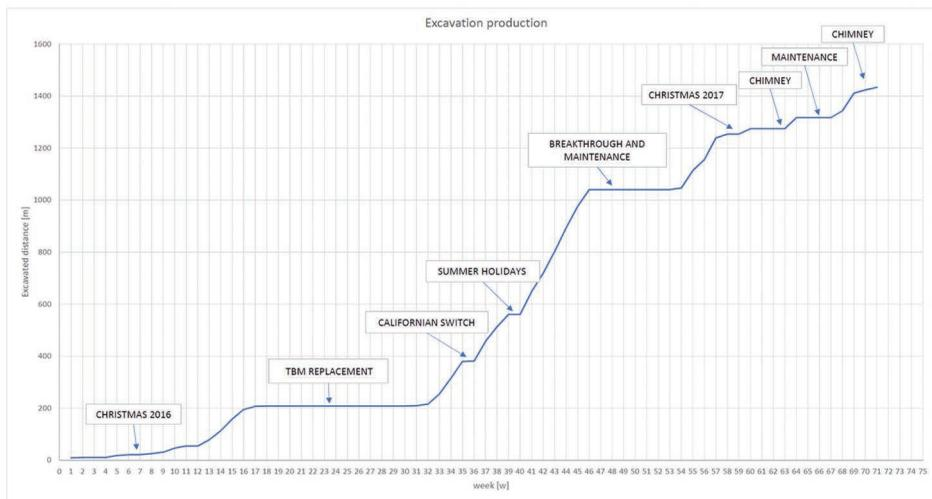
Figure 5.25 TBM’s actual daily advance records (installed rings) and main TBM’s stop reasons. (Courtesy of Geodata Engineering SpA.)
