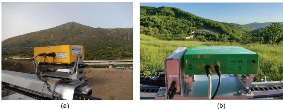
Figure 5.7 Type of terrestrial interferometer. (Courtesy of NHAZCA S.r.l.)
