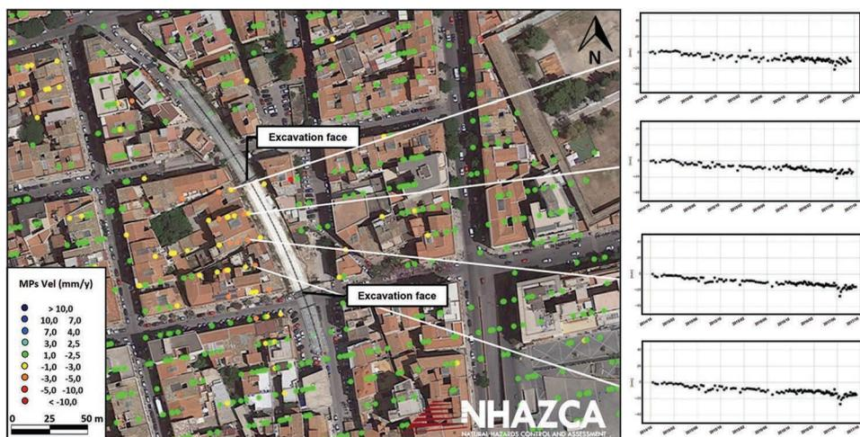
Figure 5.8 Example of settlement monitoring by satellite Interferometry.
