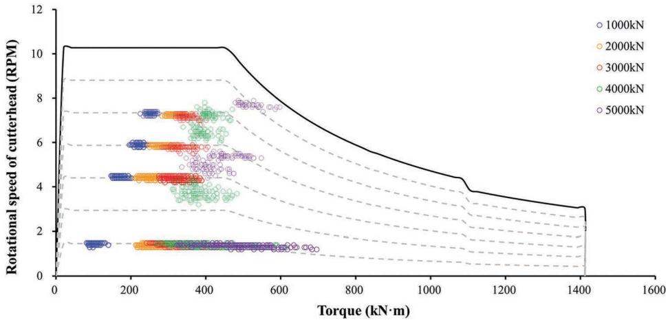
Figure 5.26 TBM's cutter head drive capacity is expressed by the relationship between torque and rotation speed (Kim, 2020).
