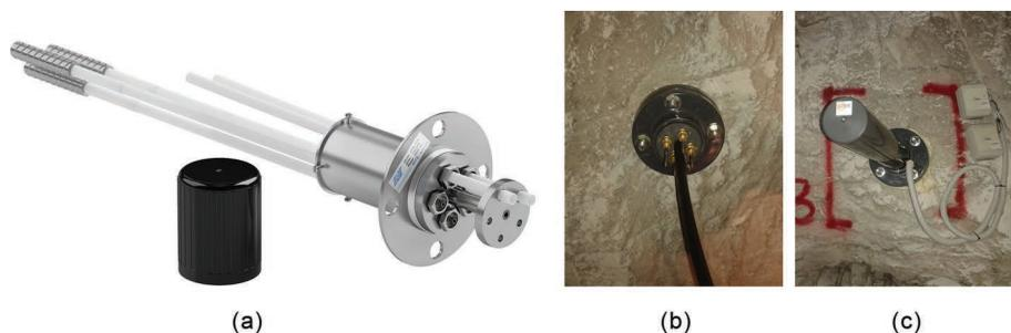
Figure 5.14 Type of a rod MPBX (a) and example of an application in a tunnel with wireless automatic datalogger (b and c). (Courtesy of Encardio Rite Ltd. and GD Test S.r.l.)
