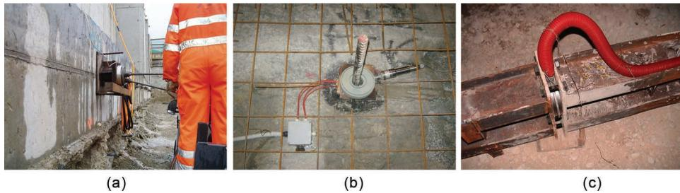
Figure 5.18 Example of different types of load cells and their application. (Courtesy of GD Test srl and Gestecno S.r.l.)
