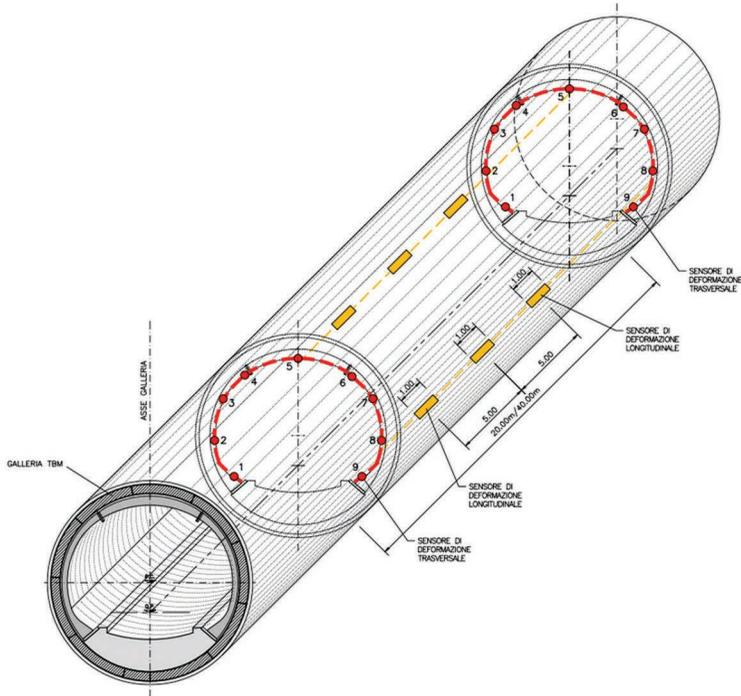
Figure 5.17 Type of optical strain gauge and example in tunneling application for convergence/section deformation and long-base longitudinal deformation sensors. (Courtesy of Smartec.)
