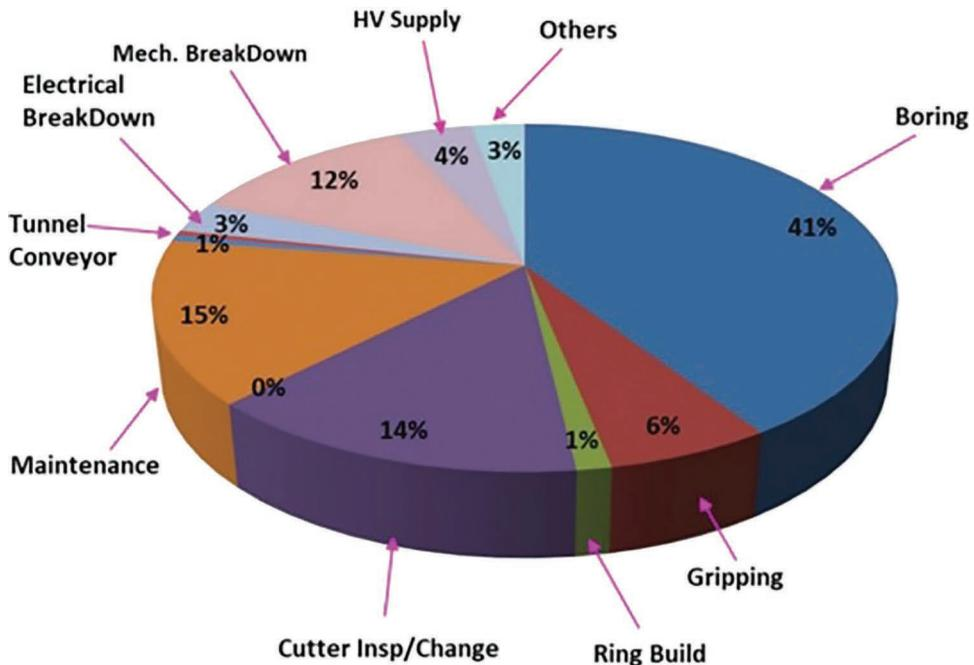
Figure 5.40 Example of an open TBM utility pie chart (Brox, 2020).
