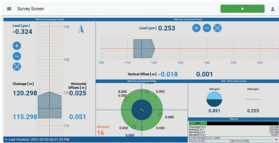
Figure 5.31 Example of screw display showing tunnel axis spatial position. (Courtesy of TACS Gmbh.)
