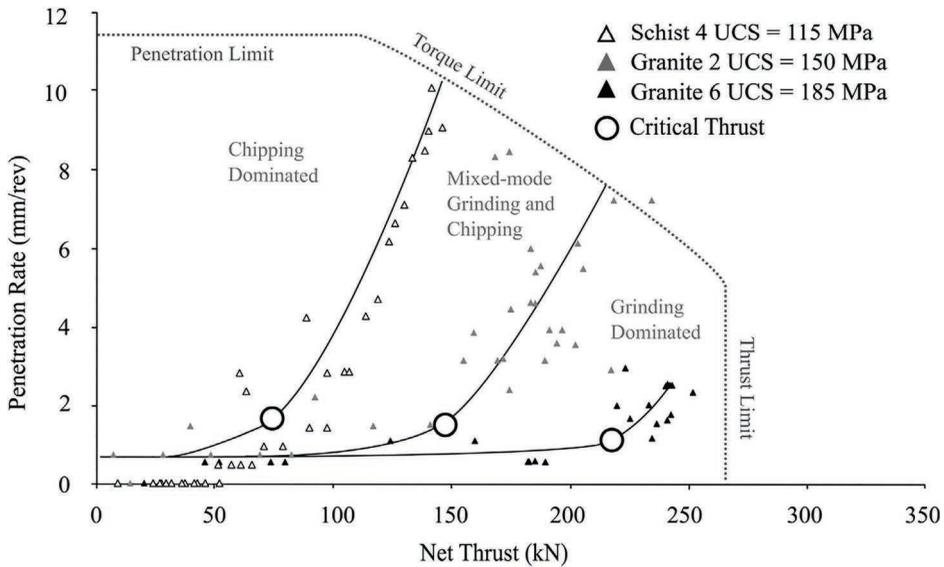
Figure 5.28 Curves cutter head thrust: penetration deriving from laboratory tests for some lithologies (Villeneuve, 2017).
