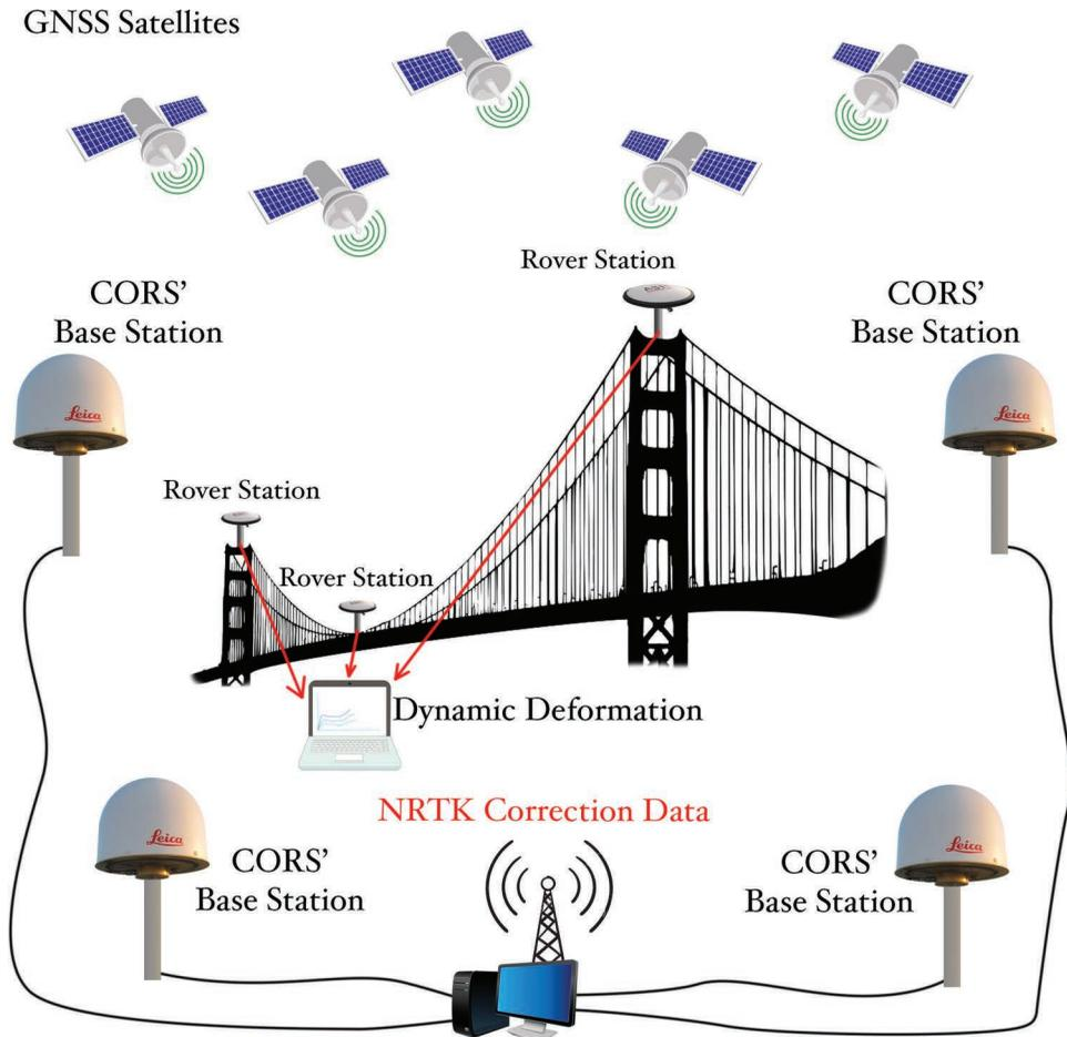
Figure 5.4 Layout of a GNSS monitoring system. (Courtesy of Leica Geosystems AG.)
