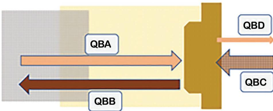
Figure 5.35 The equilibrium equation in SPB TBM tunneling.
