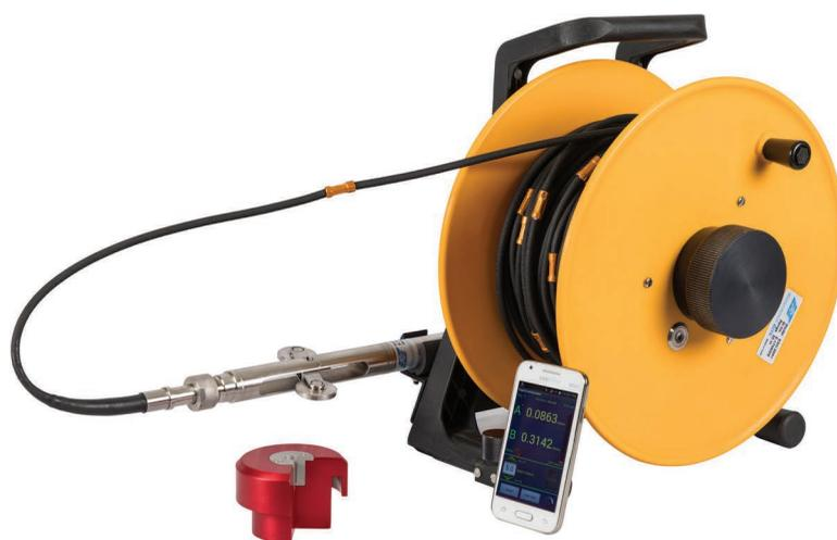
Figure 5.9 Type of removable digital system for manual measures of inclinometers. (Courtesy of Encardio rite Ltd.)
