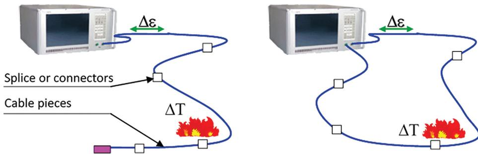
Figure 5.22 Schemes of fiber optic distributed strain/temperature sensor: (a) open configuration; (b) loop configuration. (Courtesy of Smartec.)
