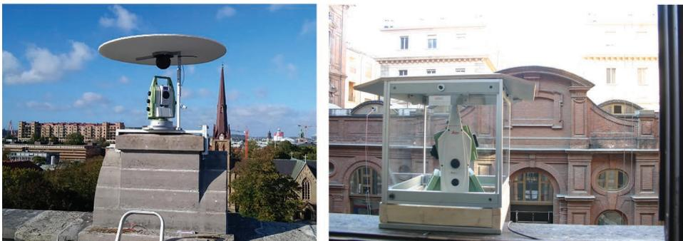
Figure 5.1 Example of ATS installed in a fixed and protected monitoring location. (Courtesy of Leica Geosystems AG.)
