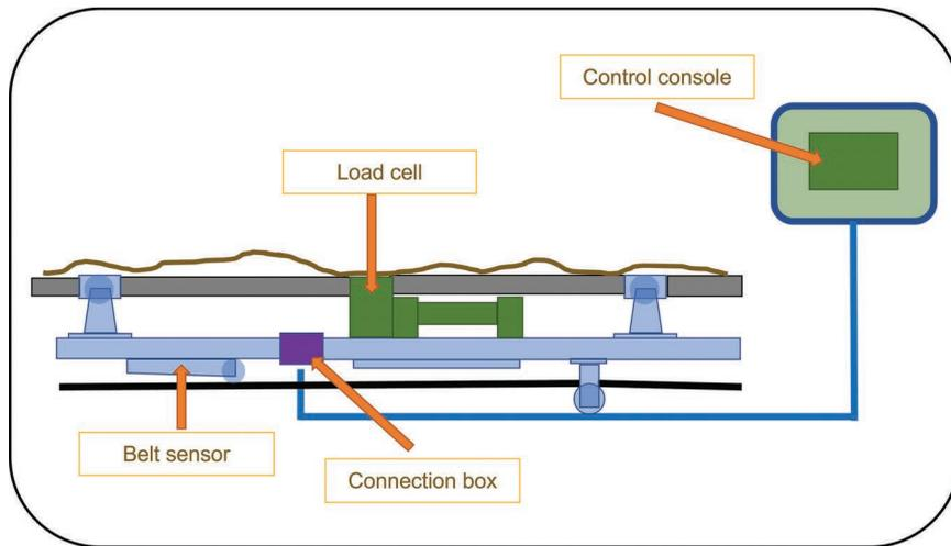
Figure 5.34 The principal components of a weighing belt conveyor system. (From <https://www.coalhandlingplants.com/belt-weigher-or-belt-scale/>.)
